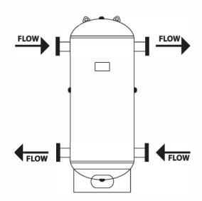
$\frac{3 \text{ X } (900,000-0)}{20 \text{ X } 500} = \frac{2,700,000}{10,000} = 270 \text{ Gallon CBTR Hot Water Buffer Tank Required}$
