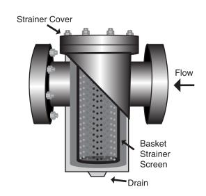
Straining of the pipeline flow is accomplished via a perforated or mesh lined basket, internal to the strainer. In general, the size of the basket perforation should be slightly smaller than the smallest debris particle to be removed. If the basket perforation is undersized, the basket may require excessive cleaning. Conversely, if the basket perforation is oversized, unwanted debris may be permitted to flow through the pipeline, possibly damaging downstream equipment.
